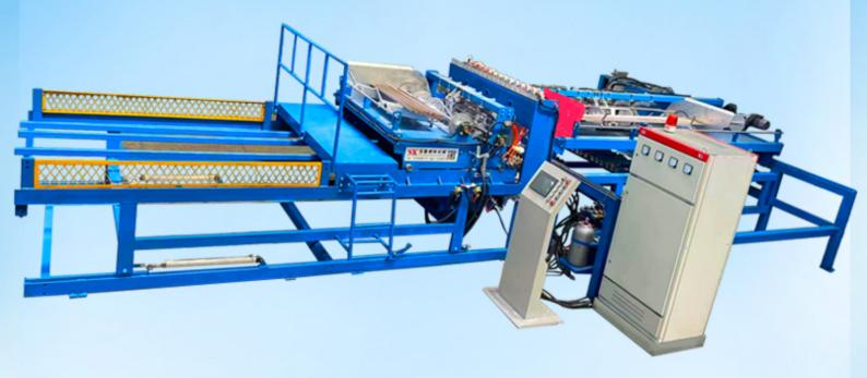
Operation system: PLC programmable controller Dynamic system: pneumatic-electric mixed
